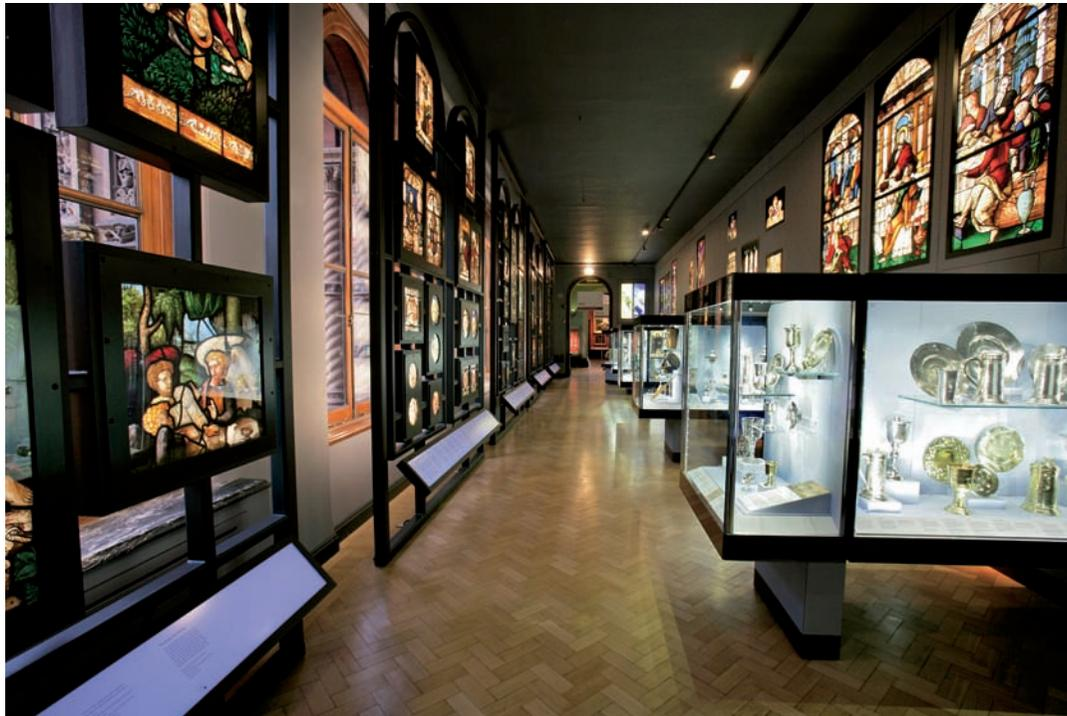
**The V&A's insistence on retaining views to the garden led VBK to use LEDs instead of daylight to illuminate the stained glass exhibits**
